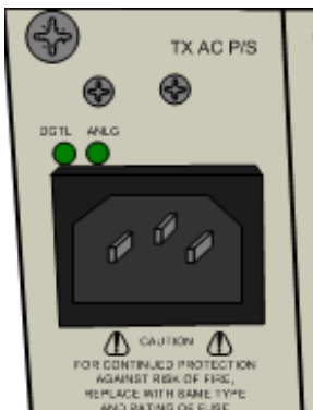
Figure 4: Power Source Connection
